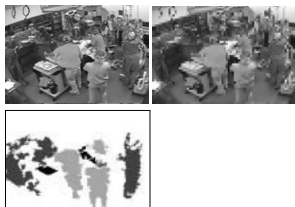
Figure 3. Image display options. Top left: original video image. Top right: corresponding pixelated image. Bottom : corresponding cartoon abstraction image. Note for the cartoon abstraction image, the people working in the OR were represented as blobs in different colors. When viewed overtime, cartoon images allow identification of some of the activities.
