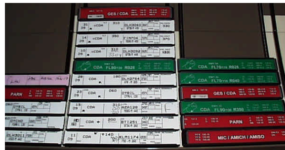
Figure 3: A strip rack with en route strips for aircraft in an en route sector.
