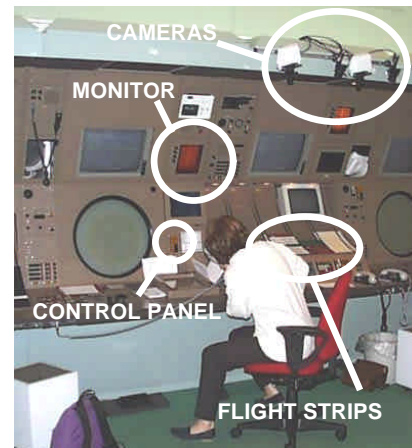
Figure 5: En route controller handling both the radar and the planner positions in ACC East. The cameras are aimed at flight strips for aircraft approaching Copenhagen Airport from the south.
